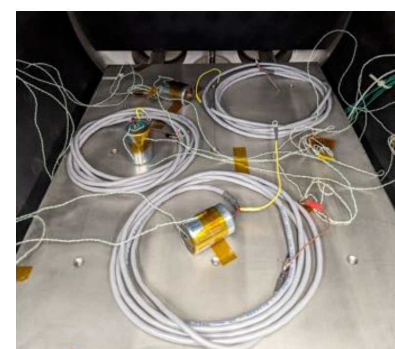
Environment testing of the seismic sensors @ ISAE-SUPAERO
